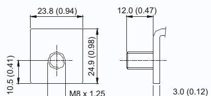
Terminal Hardware Initial Torque: 10.0Nm ±5%
